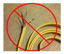
11. All wire splices must be properly connected inside an electrical box or approved enclosure.
